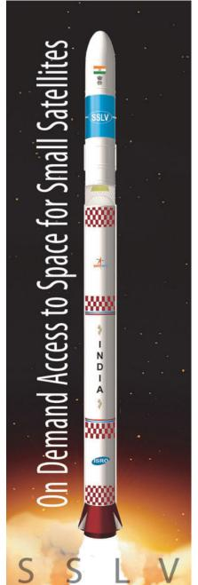
• SSLV is the new small satellite launch vehicle developed by ISRO to cater the launch of small satellites up to 500 kg to Low Earth Orbits on 'launch-on-demand' basis.
